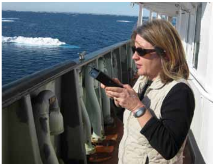
Figure 5. During a beautiful day in the high arctic, PolarTREC teacher Gerty Ward takes a reading of the solar radiation intensity with a Microtops photometer. Sunlight in the Arctic has an important contribution to the Earth's energy budget, and NASA will use the data collected by the photometer to verify satellite data.
