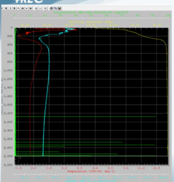
Conductivity-Temperature-Depth (CTD) Trace - This is an electronic measurement made in the water. Water samples also collected from this device
