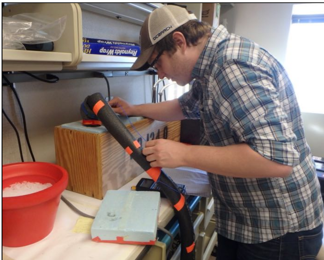
Graham Lobert and the thermal block the team designed to create a water temperature gradient.
