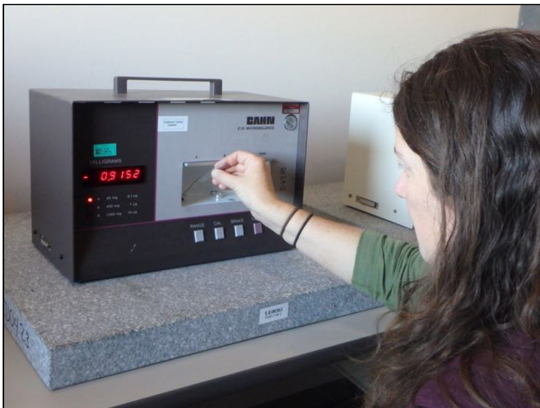
Amy Osborne uses an electrobalance to determine the weight of eggs. Photo by Aaron Toh.
