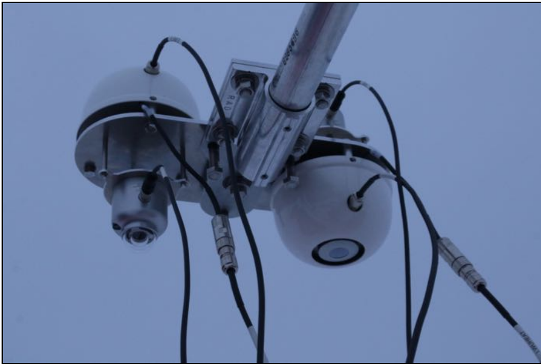
This radiometer measures incoming and outgoing shortwave and longwave radiation.
