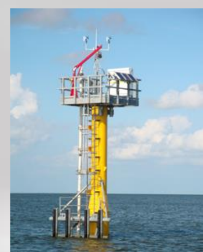
A water level observation station, part of the National Water Level Observation Network. Photo courtesy of NOAA.
