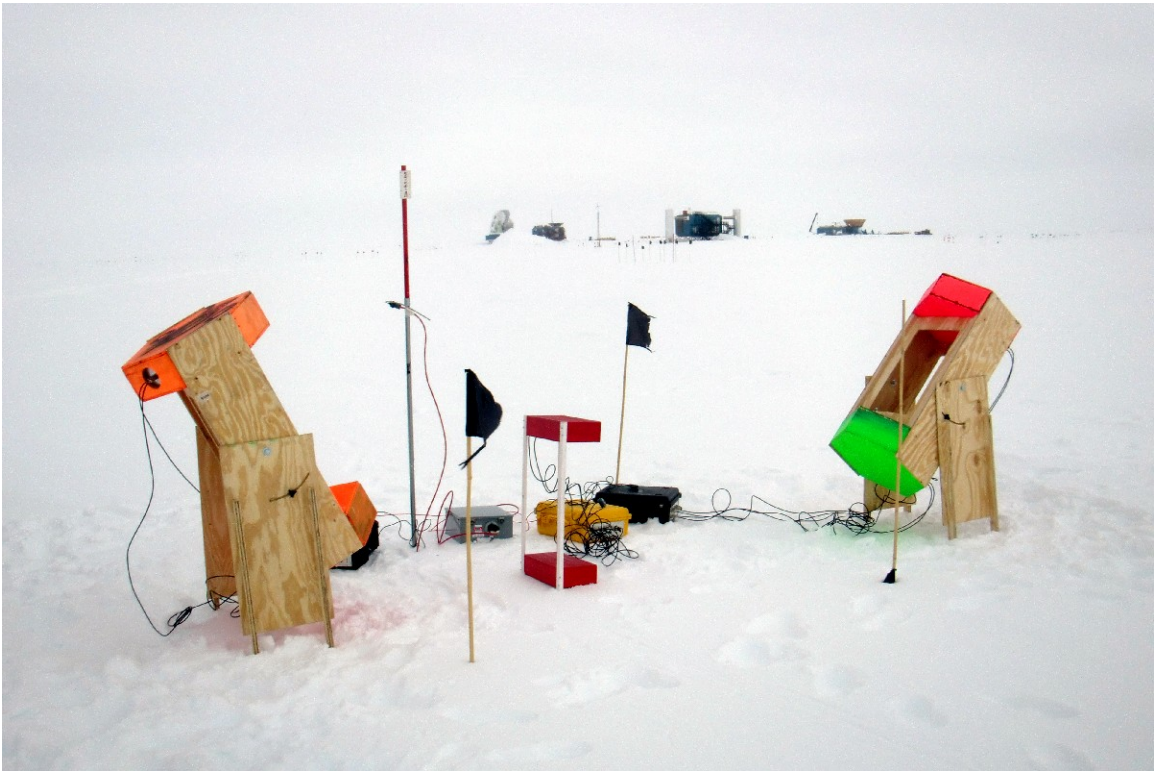
The sensors are attached to the wooden stands, while the data acquisition modules (DAQs) are housed in the Pelican cases. The IceCube Laboratory is in the background.
