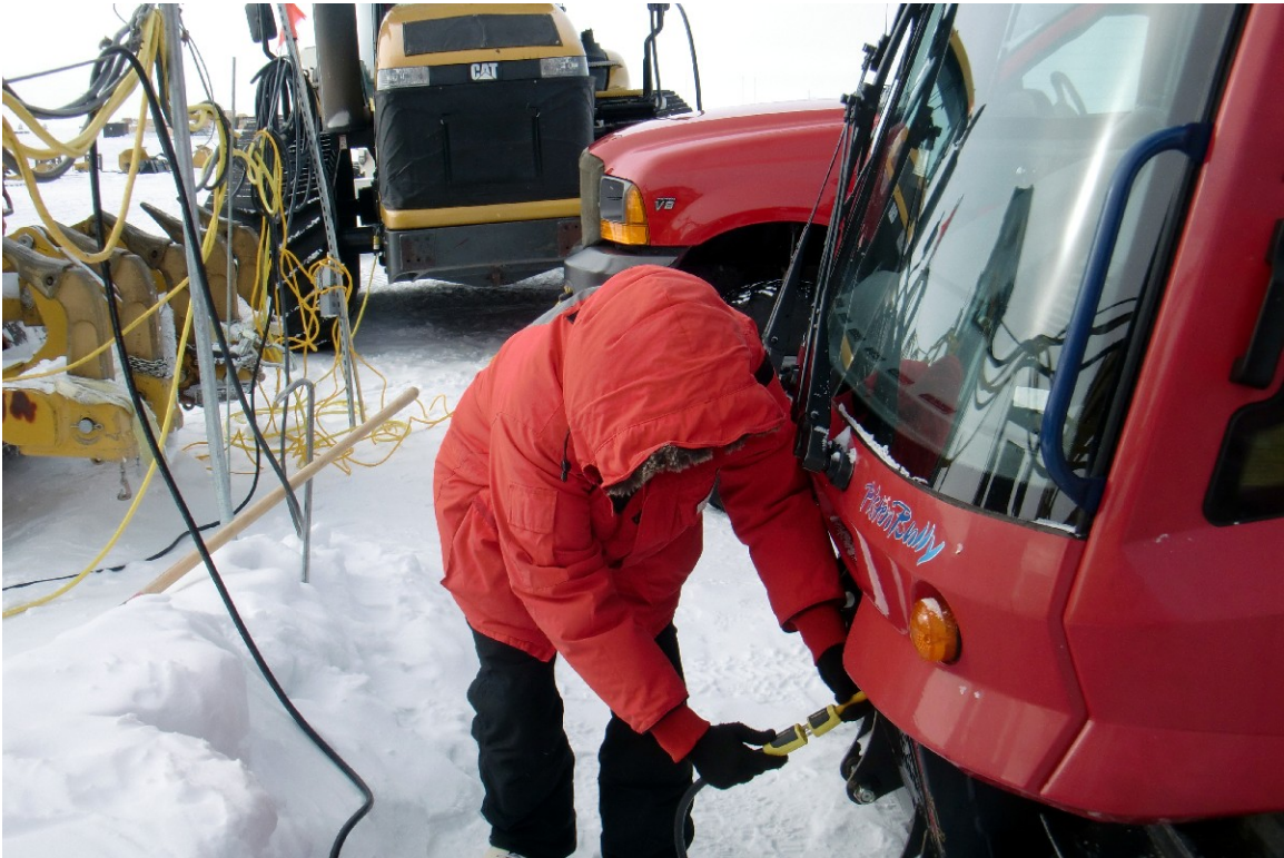
Back at the station after three and a half hours in the field. Armando is plugging in the vehicle's engine block heater.
