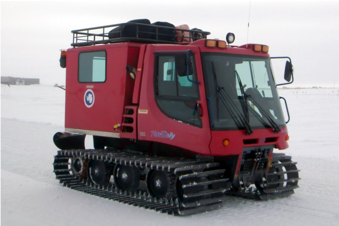
This is what the IceCube team drove in the field—a PistenBully continuous track vehicle. January 17, 2015 at 3:40 pm.
