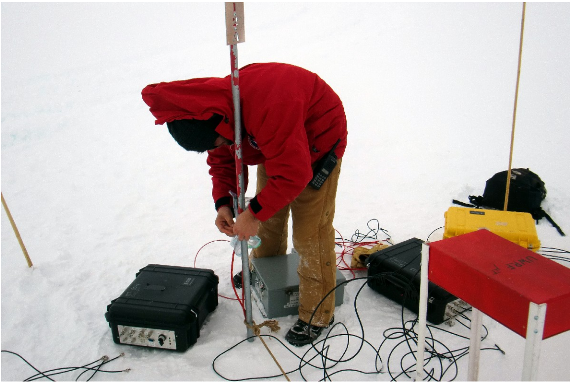
Sam while checking up the data acquisition modules (DAQs) above an IceTop station.
