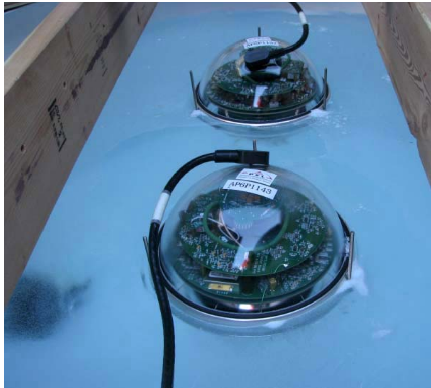
Photograph of a frozen IceTop tank ready to be closed. Credit: IceCube Collaboration.
