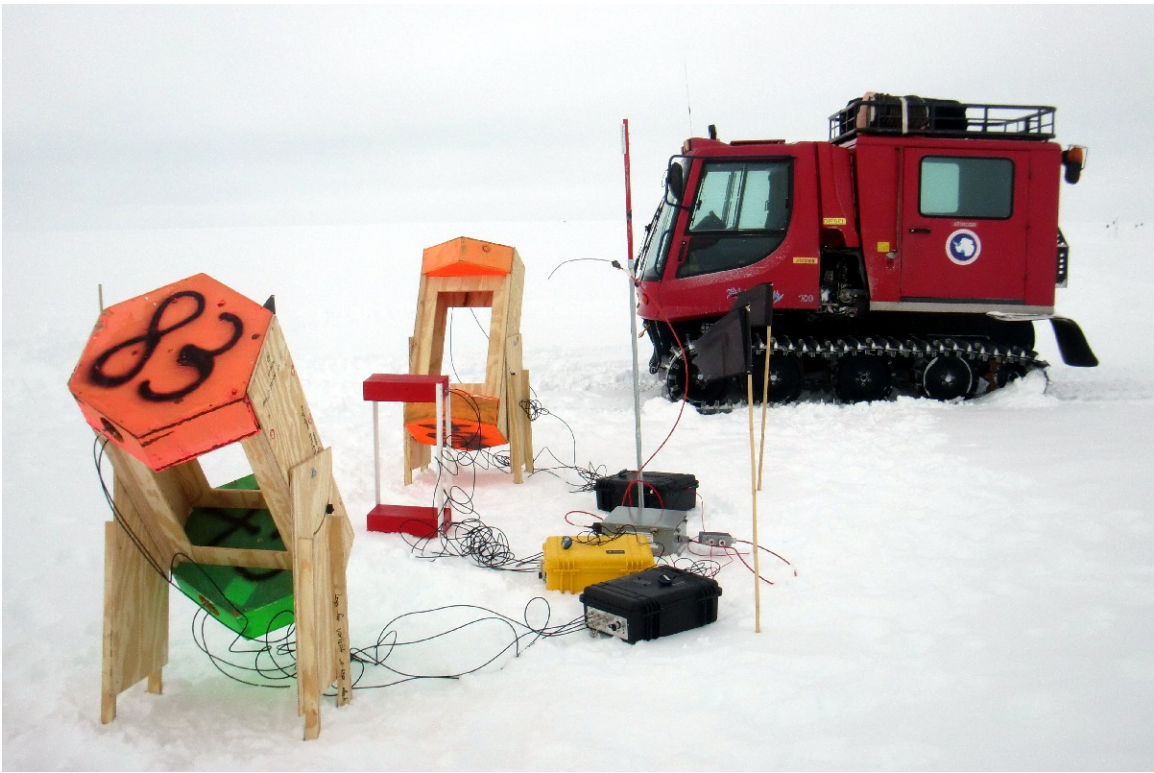
Cosmic rays sensors out in the field, right above an IceTop tank. The PistenBully vehicle that the team drove is behind.
