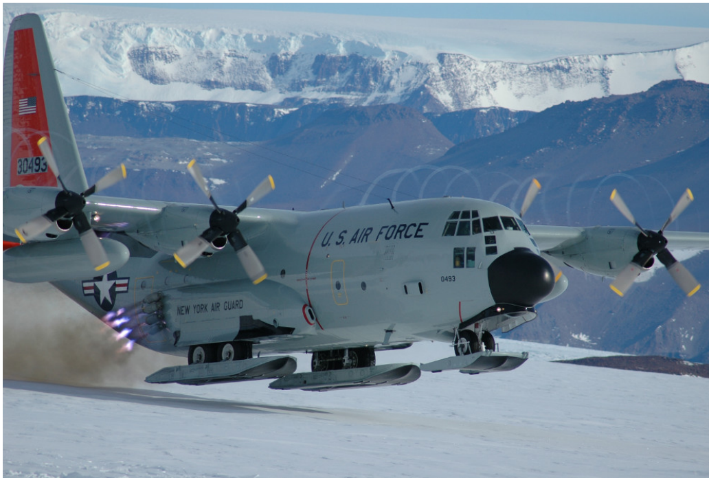
The LC-130 Hercules, a ski-equipped aircraft. Credit: Charles Kaminski, NSF (USAP Photo Library).
