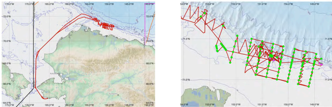
Figure 1. (Left) Cruise track from Nome AK to Nome AK. (Right) Enlargement of operating area. Track of ship is shown in red, stations are shown in green, and mooring locations are shown as the purple triangles. Saw tooth pattern along second N-S line from the east shows tacking during the strongest upwelling winds. Figures by S. Roberts (UAF).
