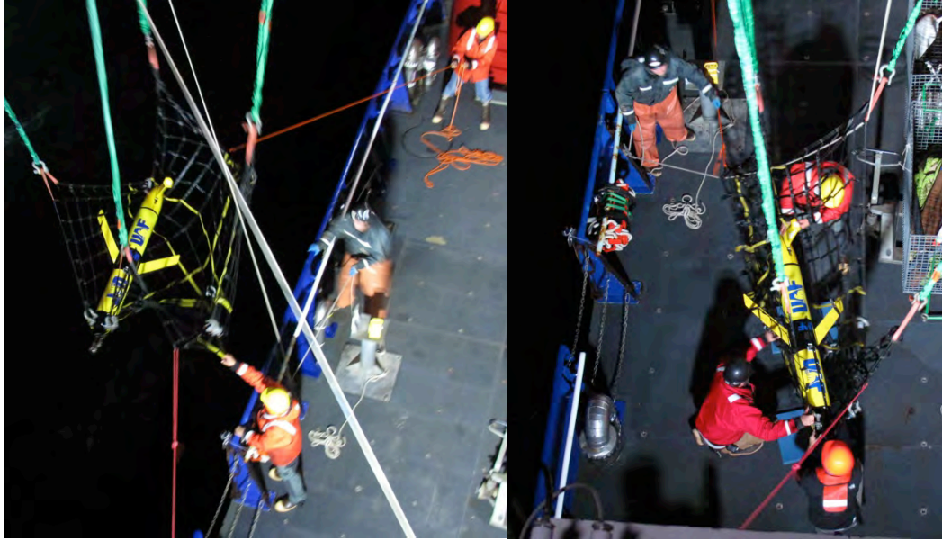
Figure 4. The glider being lifted on board (Left) and placed on the deck (Right).
