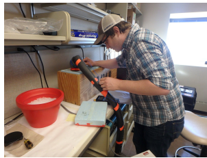
PhD student Graham Lobert observes embryos in a thermal block. A tool designed by the research team that creates a temperature gradient in water.
