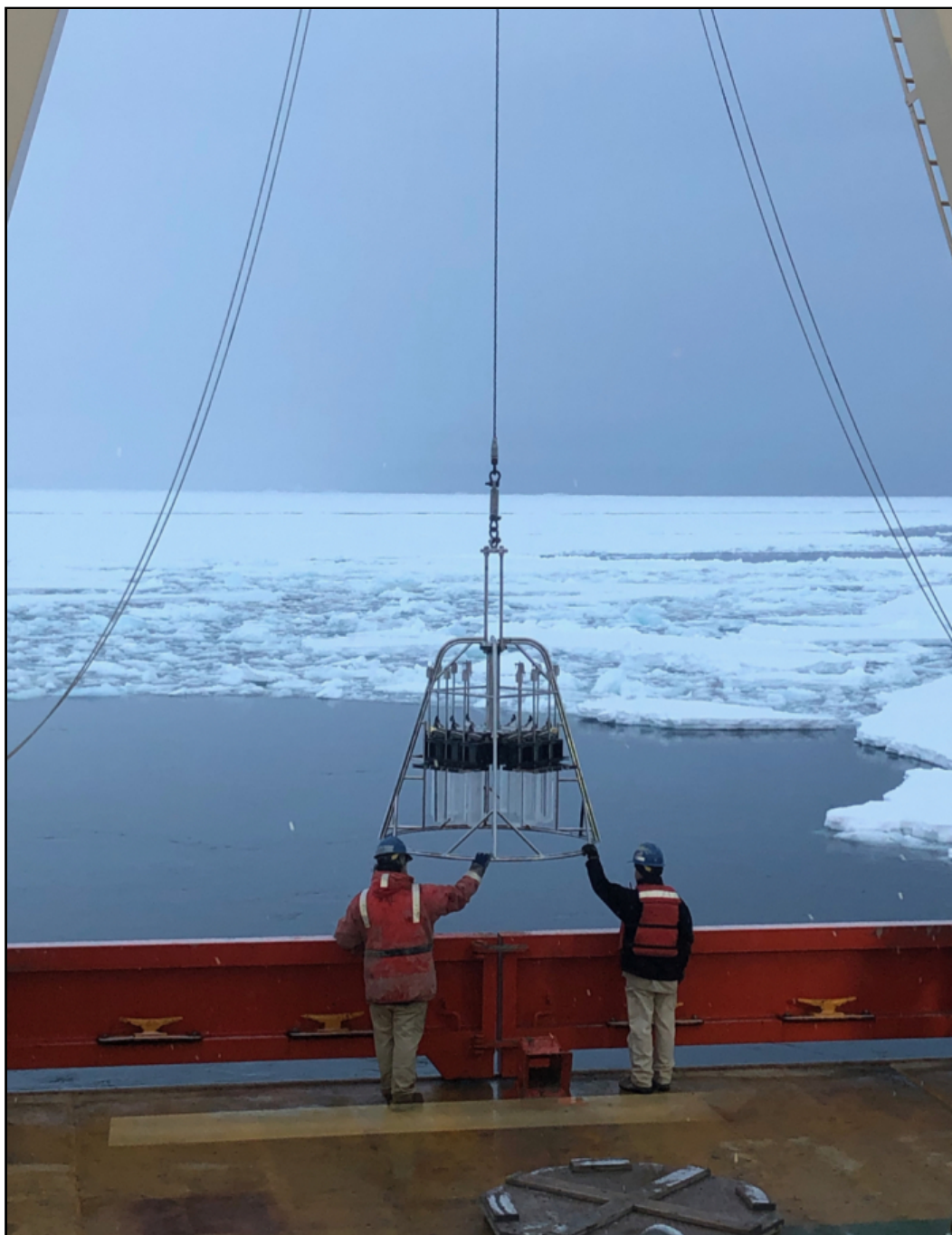
Marine Techs Richard Thompson and Chuck Holloway deploy the megacore sediment sampler over the stern of the R/V Nathaniel B. Palmer icebreaker in the Amundsen Sea off the southwest coast of Antarctica
