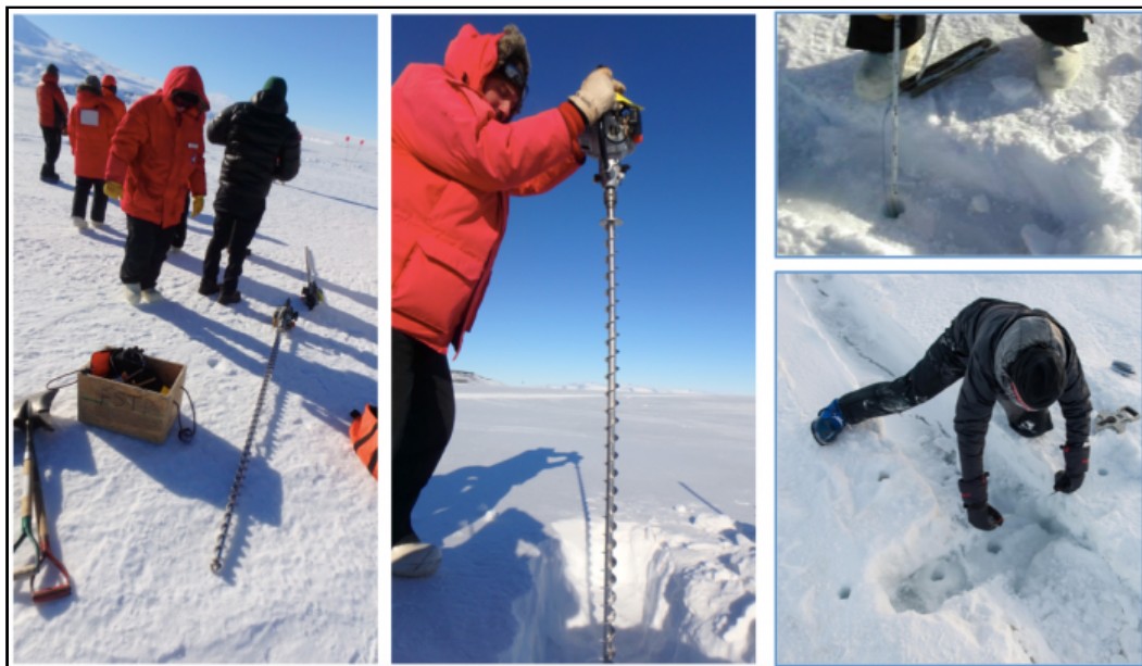
Drills with long sectional bits are used to drill through the ice so that ice thickness can be measured accurately.
