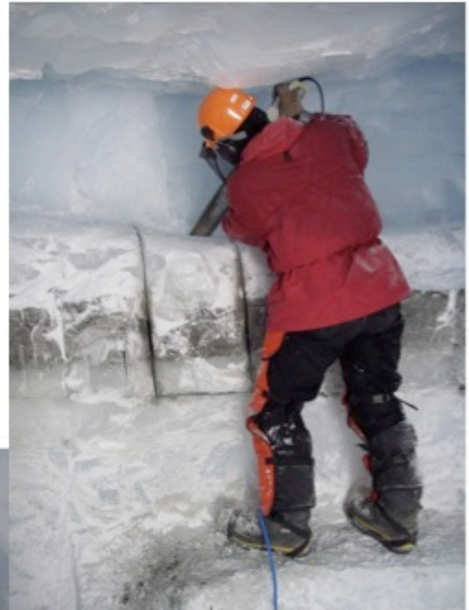
Cutting Out the Sample Blocks
