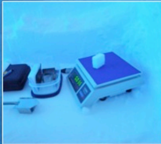
Measuring snow density to determine when the snow was deposited (winter vs. summer)
