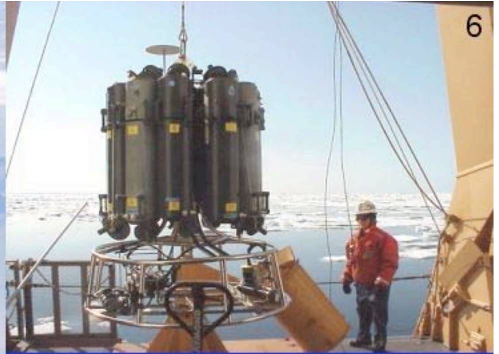
CTD (conductivity-temperature-depth) instrument, plus rosette bottles to collect seawater
