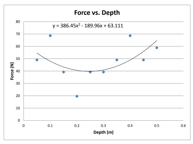
Although there is a high standard deviation, the force vs. depth generally increases as a function of depth which is generally true. Fitting the graph to a polynomial does show the decrease in force after 10 cm and then the rise again which the next graph also illustrates.
