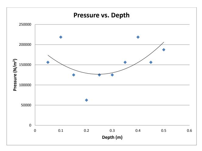
Again, pressure applied vs. depth is increasing. This of course will follow force as they are directly proportional. However, you can calculate the average pressure (or force, whichever you prefer) the skis exert on the snow and see if this value is greater or smaller than the smallest pressure the snow can withstand.
