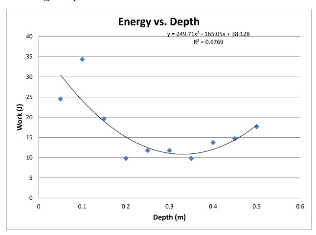
The graph above follows the F vs. Depth, but with much less scattering. Typically the snow is harder at the surface (it has a crust) and then gets softer for awhile but eventually begins to get harder as the weight of the snow compacts the snow. The graph illustrates this very well.
