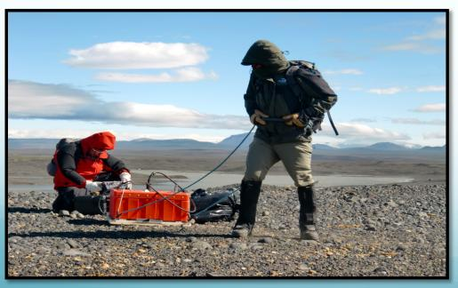
The GPR unit was used by the team to determine the structure of subsurface till layers composing the drumlins. The GPR was pulled across the drumlins while collecting data. It was also used on the glacier's ice margin to get information about how the drumlins emerge from underneath the glacier.
