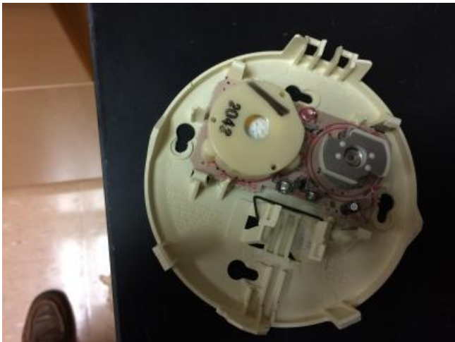
Smoke detector alpha source.
