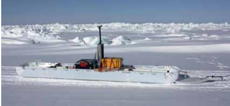
Electromagnetic device for measuring ice thickness
