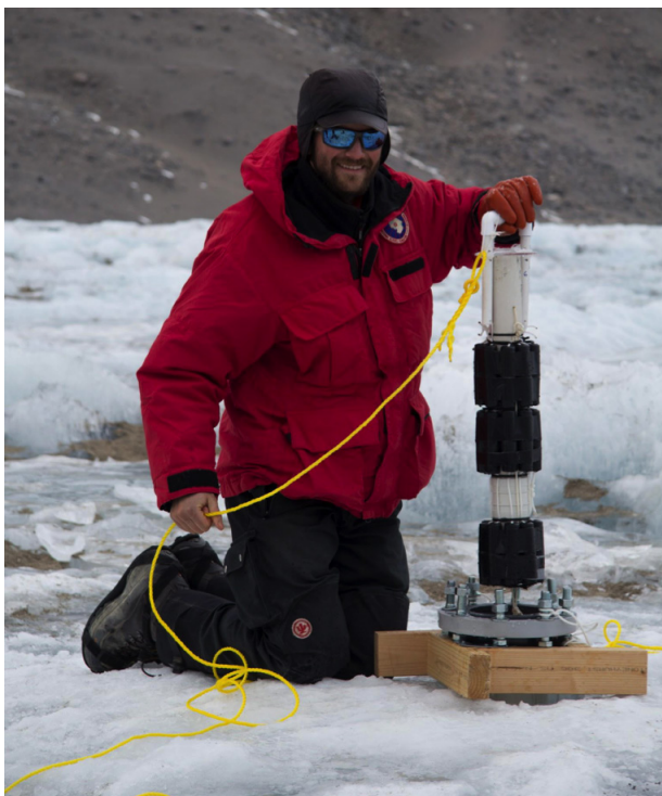
Tyler Mackey installing a sediment trap.
