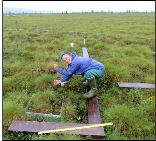
Karen Temple-Beamish forces a thin rod into the tundra to determine the depth to permafrost. Photo by Karen Temple-Beamish.
