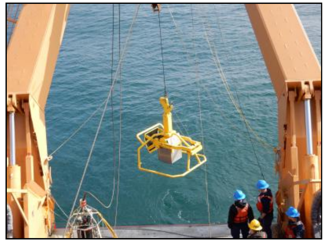
The crew prepares to deploy the box corer aboard the USCGC Healy icebreaker in the Bering Sea. Photo by Sandra Thornton
