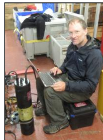
Mike DeGrandpre (UM) downloads data from a SAMI after a year long deployment on a mooring in the Beaufort Sea.
