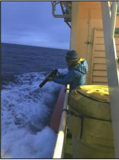
Launching the XPT to measure temperature and depth while crossing the drake passage.
